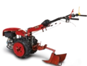
Assolcatore professionale (accessorio) Professional furrower (implement)
