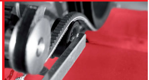
Cinghia dentata in kevlar: dura il triplo di quelle normali! Kevlar toothed belt: last three time longer than normal ones!
